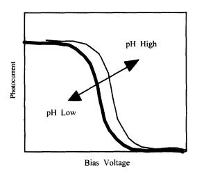
Fig. 3. Relations between the bias voltage/photocurrent and the pH value.
