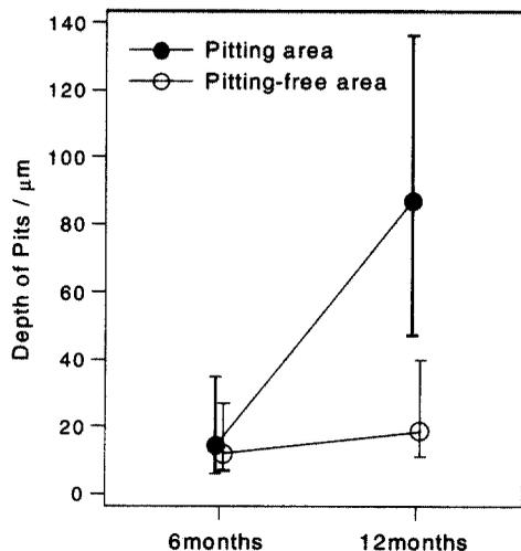
Fig. 8. Time evolution of depth of pits in pitting and pitting-free area.
