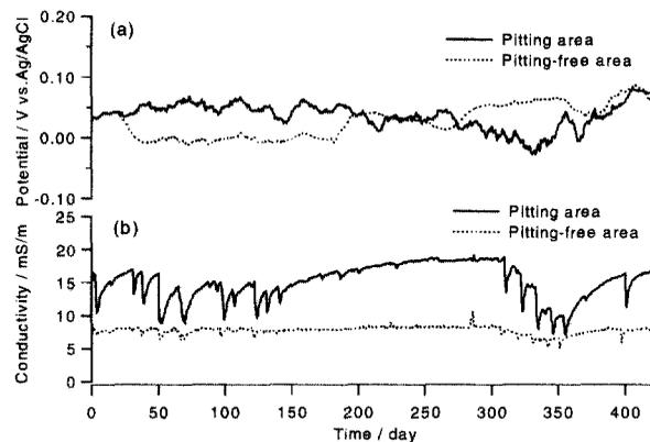
Fig. 3. Corrosion potential-time curves of copper tubes and electric conductivity-time curves of tap water in pitting and pitting-free area: (a) Corrosion potential, (b) Electric conductivity.
