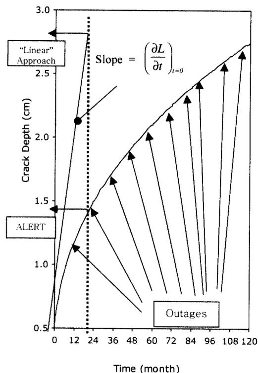
Fig. 2. Illustration of the nonlinearity of the accumulated damage and inadequacy of the linear approach for extrapolating crack propagation for future operating periods (regular and identical outages and fuel cycles).
