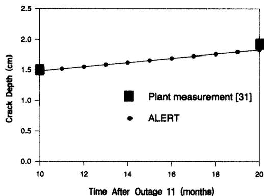
Fig. 4. Depth of the crack in the H-3 weld monitored by Tang, et al.<sup>31)</sup> in an operating BWR as a function of time after Outage 11. The calculated and measured depths at ten months were made to coincide by adjusting the initiation time, so that only the comparison at 20 months has value.
