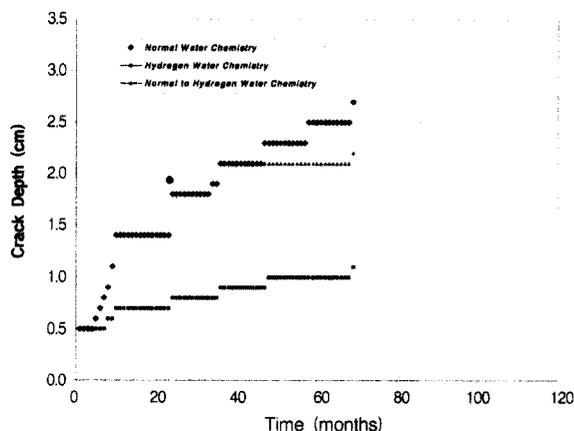
Fig. 3. Predicted histories of a growing crack in the core shroud of an operating Boiling Water Reactor as a function of pre-conceived future operating histories. Note that the discontinuities in the crack length arise from changes in crack growth rate during outages (irregular outages).
