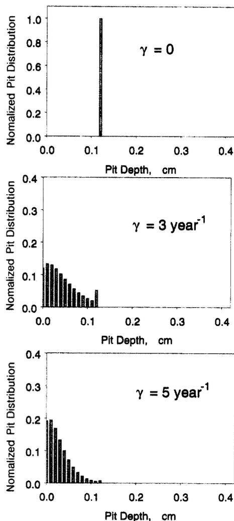
Fig. 1. Influence of the value of  $\gamma$  on normalized pit distribution for  $C_{\text{NaCl}} = 0.1 \text{ mol/L}$ ,  $E_{\text{corr}} = -0.384 \text{ V (SHE)}$ ,  $\text{pH} = 7$ ,  $T = 25^\circ\text{C}$ , and  $t_{\text{obs}} = 1 \text{ year}$ .
