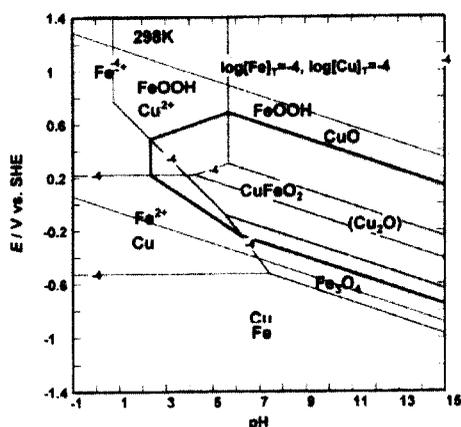
Fig. 9. E-pH diagram for Fe-Cu system.
