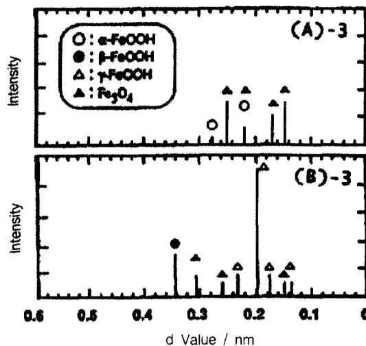
Fig. 6. Transmission electron diffraction of (A) Ni- and (B) Co-bearing steels. Selected areas for the diffraction corresponded to those of Ni- and Co-enrichment.
