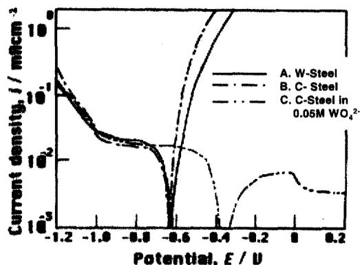
Fig. 8. Polarization curves for W-bearing steel in NaCl solution and 0.05 M  $\text{WO}_4^{2-}$  - NaCl solution.
