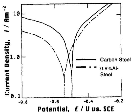
Fig. 7. Polarization curves for an Al-bearing steel obtained after the treatment of 8 cycles of wet/dry corrosion test.
