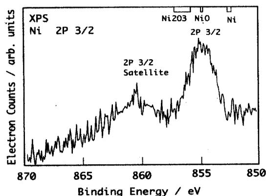
Fig. 4. XPS analysis of the rust on Ni-bearing steel. Ni in the rust in the bivalent state (Ni(II)).
