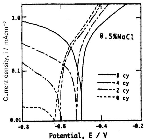
Fig. 1. Polarization curves of rusted steels processed by wet/dry/rinse cycle. Cathodic current markedly increases with increase in number of corrosion cycles.
