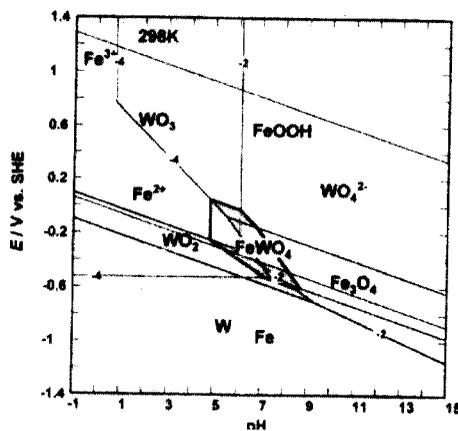
Fig. 12. E-pH diagram for Fe-W system.
