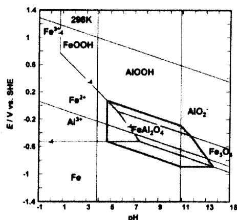
Fig. 11. E-pH diagram for Fe-Al system.
