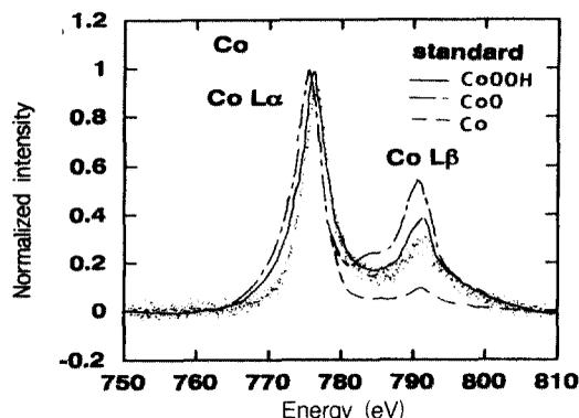
Fig. 5. XPS spectra for the rust of a Co-bearing steel and reference Co Compounds
