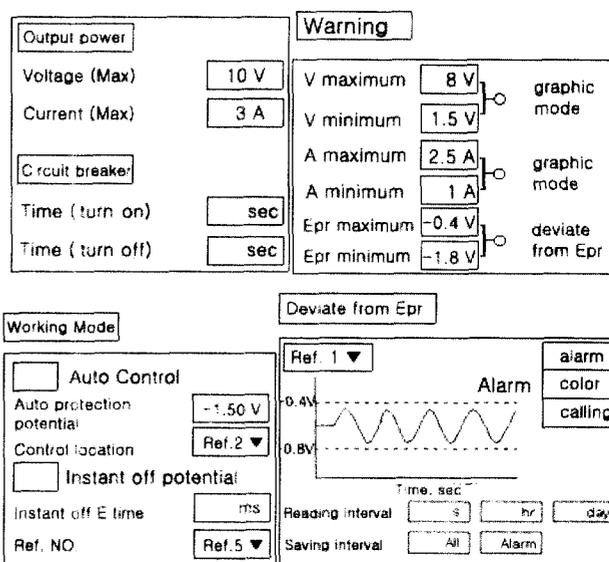
Fig 6. Remote monitoring and controlling system for electrochemical cathodic protection
