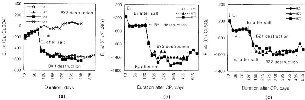
Fig. 2. Open circuit potential (a) and protection potential (b, c) of specimen B in salt water
