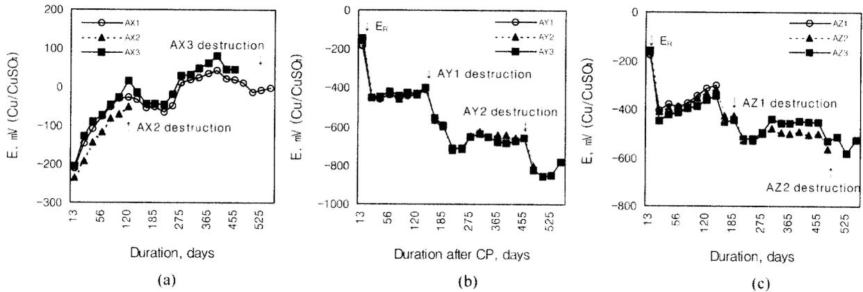
Fig. 1. Open circuit potential (a) and protection potential (b, c) of specimen A in air
