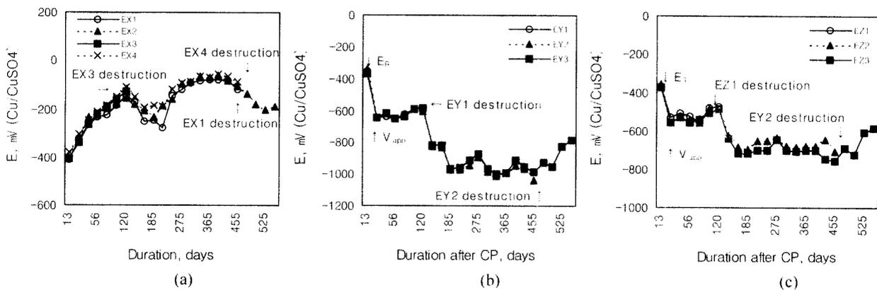
Fig. 3. Open circuit potential (a) and protection potential (b, c) of specimen E in air
