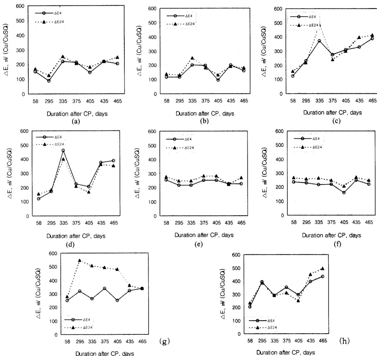
Fig. 5. Instant on-off potentials; (a)(c)(e)(g) used mesh type anode, (b)(d)(f)(h) used ribbon type anode, (a)(b)(e)(f) are tested in air, (c)(d)(g)(h) are tested in salt water
