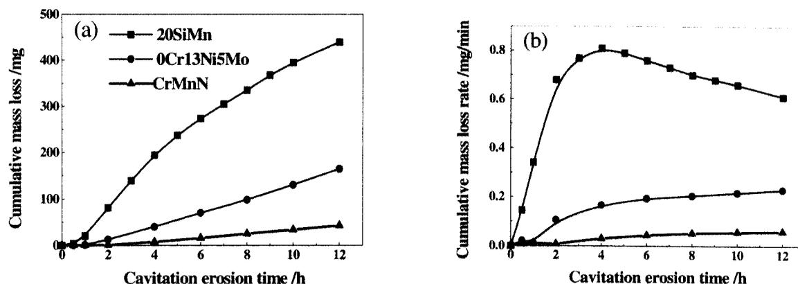
Fig. 1. Cavitation erosion behaviors of 20SiMn, 0Cr13Ni5Mo and Cr-Mn-N in distilled water.
