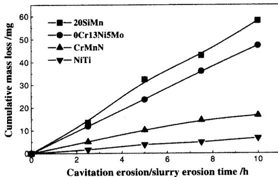
Fig. 9. The comparison of the combined action of slurry erosion and cavitation erosion of four materials in tap water containing  $0.25 \text{ kg/m}^3$  silica sand (200-300mesh) at 18m/s obtained by rotating disk rig.
