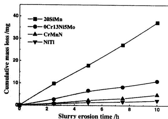
Fig. 7. The comparison of slurry erosion behaviors of four materials in tap water containing 0.25 kg/m<sup>3</sup> silica sand (200-300mesh) at 18m/s obtained by rotating disk rig.
