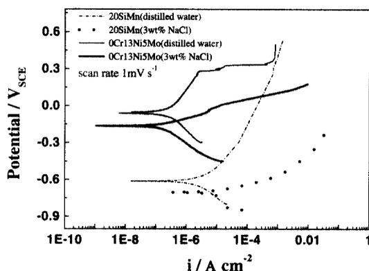
Fig. 6. Potentiodynamic polarization curves for 20SiMn and 0Cr13Ni5Mo in distilled water and 3wt%NaCl solution under quiescent condition at 27°C.
