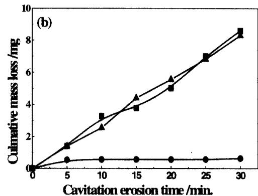
Fig. 5. Effects of solid particles and corrosion on cavitation erosion behaviors of 20SiMn and 0Cr13Ni5Mo. (a) 20SiMn (b) 0Cr13Ni5Mo
