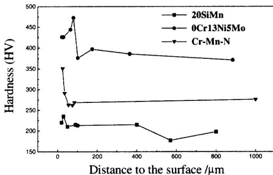
Fig. 4. Hardness of 20SiMn, 0Cr13Ni5Mo and Cr-Mn-N after 3-hour cavitation erosion test in distilled water.
