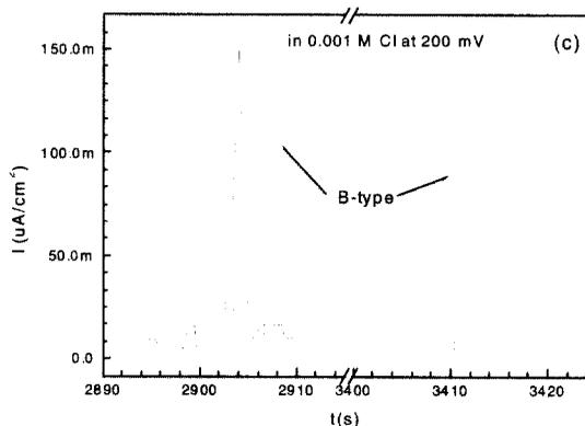
**Fig. 4.** Typical current transient generated by metastable pitting of alloy 690 in deaerated NaCl solutions at 90°C under potentiostatic conditions, (a): in 1 M Cl at 0 mV, (b) in 0.1 M Cl at 0 mV, (c) in 0.001 M Cl at 200 mV.
