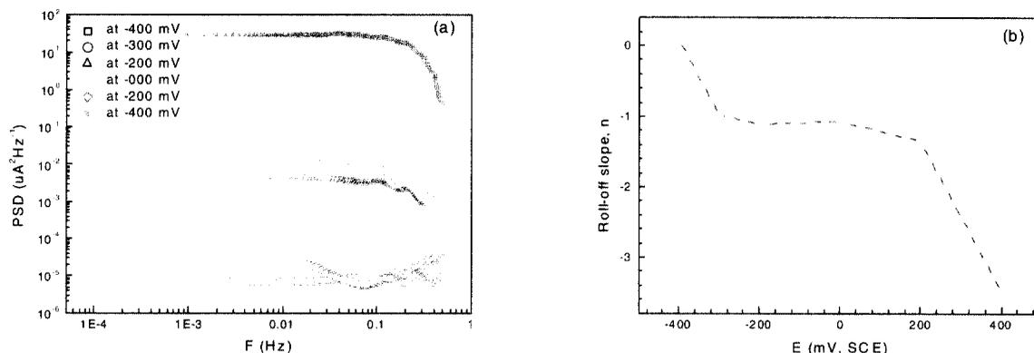
**Fig. 9.** Current PSD and roll-off slopes plots of alloy 690 in deaerated 0.01 M Cl<sup>-</sup> solutions at various polarization potentials in deaerated solutions at 90°C, (a)PSD, de-trend DC drift, MEM plot, order 10, hanning window, data obtained from Figure 6 starting at 1024 to 2048, (b) roll-off slopes
