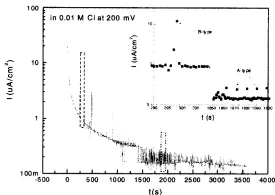
**Fig. 3.** Typical current transient of alloy 690 in deaerated 0.01 M NaCl solution at 90°C at 200 mV (SCE), sampling frequency: 1Hz. Also shown the typical single transient (me-tastable pitting), A-type: fast current rise and a fast fall, B-type: slow current rise followed a quick fall
