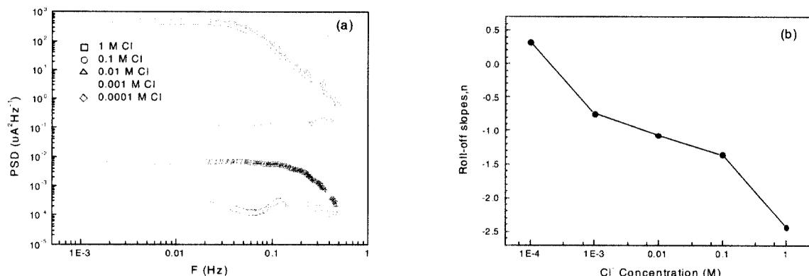
**Fig. 8.** Current PSD and roll-off slopes plots of alloy 690 in deaerated various Cl<sup>-</sup> solutions at 0 mV in deaerated solutions at 90°C, (a)PSD, de-trend DC drift, MEM plot, order 10, hanning window , data obtained from Figure 5 starting at 1024 to 2048 (in 1 M Cl, from 1 to 1024)
