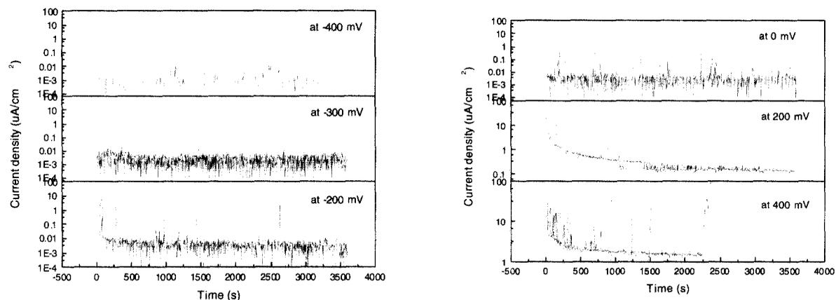
Fig. 6. Time series showing the effect of polarization potential on the current spikes of metastable pitting in deaerated 0.01 M NaCl solutions at 90°C
