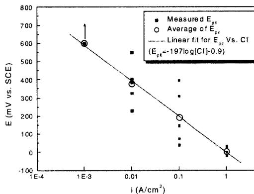
**Fig. 2.** Epit of alloy 690 as function of Cl<sup>-</sup> concentration in deaerated solutions at 90°C, data from the anodic polarization curves (at least 3 identical experiments at each concentration, in 0.001M Cl<sup>-</sup> and 0.0001 M Cl<sup>-</sup> solution, no pitting)
