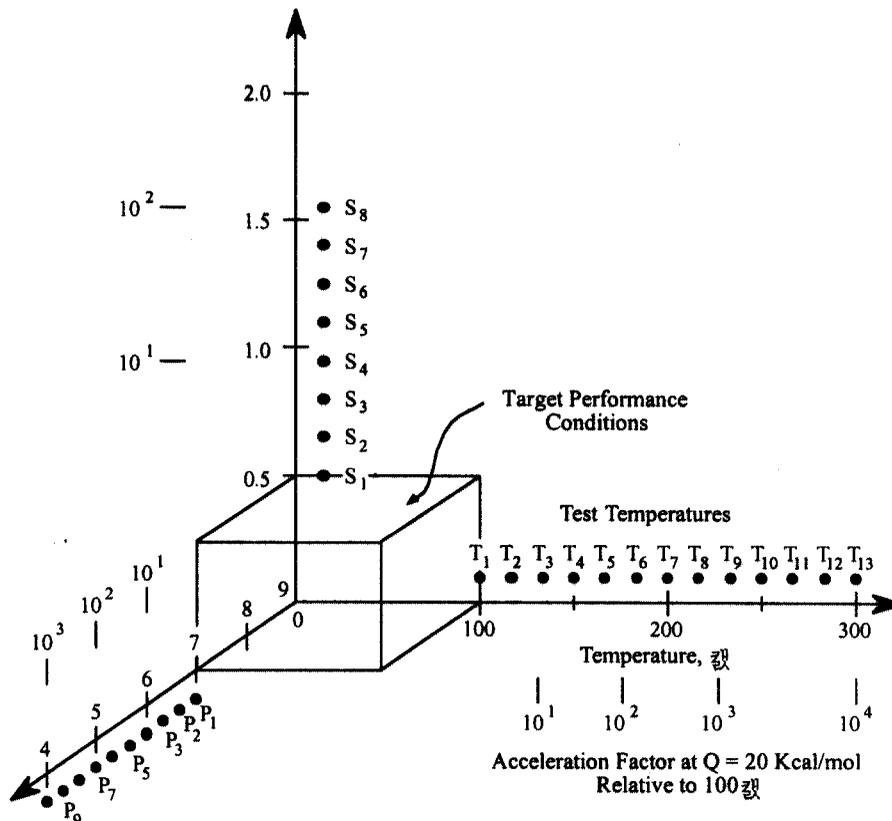
Fig. 16. Schematic view of accelerating variables of temperature, stress, and pH relative to a box of expected conditions. Each coordinate shows the magnitudes of acceleration.
