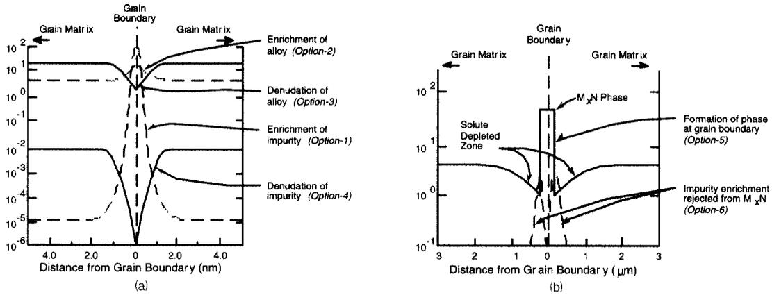
Fig. 6. Concentration vs. distance from the grain boundary for several cases. (a) Atoms adsorbed or rejected. (b) Compound formed requiring sources from surroundings. From Staehle.<sup>12)</sup>
