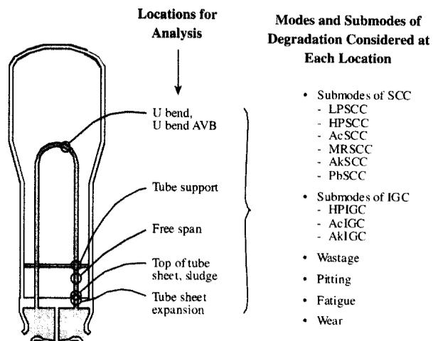
Fig. 3. Schematic view of steam generator from a pressurized water nuclear reactor with different locations for analysis and the possible modes and submodes for a single tube. From Staehle.<sup>1)</sup>
