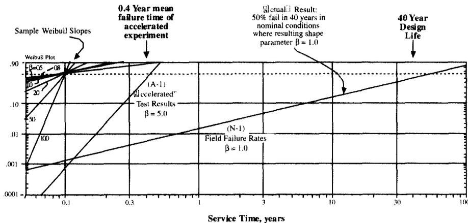
Fig. 18. Schematic comparison of hypothetical actual field results with hypothetical accelerated testing using cumulative distribution versus time. N-1 with  $b=1.0$  is the nominal field failure rate. A-1 with  $b=5.0$  corresponds to an accelerated test. N-2 is the desired field failure rates that does not exceed 0.001 cumulative failures in 40 years. A-2 has the same slope as A-1 for a mean life of 40 years; A-3 has the same slope but with 0.001 failures in 40 years.<sup>8)</sup>
