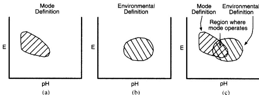
Fig. 11. Schematic view of the superposition process. (a) Mode definition. (b) Environmental definition. (c) Comparison of mode and environmental definitions. From Staehle.<sup>16)</sup>
