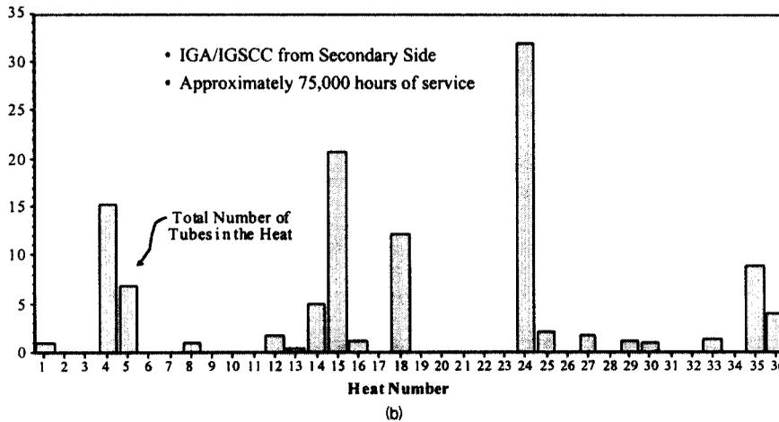
Fig. 7. Percent of tubes affected by corrosion versus heat number for steam generators at a single plant. Primary and secondary sides are not from the same sets of steam generators. Numbers at the top of each bar indicate number of tubes from each heat. (a) LPSCC on primary side at roll transitions. (b) IGA/IGSCC from secondary side. From Scott.<sup>13)</sup>
