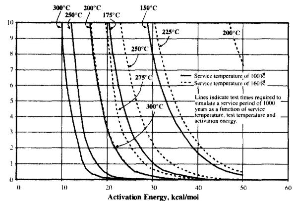
Fig. 17. Time for testing versus activation energy for different testing temperatures where the objective is determining life at 1000 years for the cases where surface temperatures are either 100 or 160°C.
