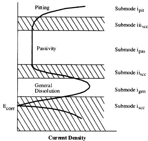
Fig. 9. Schematic view of regions of SCC, general dissolution, pitting and passivity related to a polarization curve. From Staehle.<sup>18)</sup>
