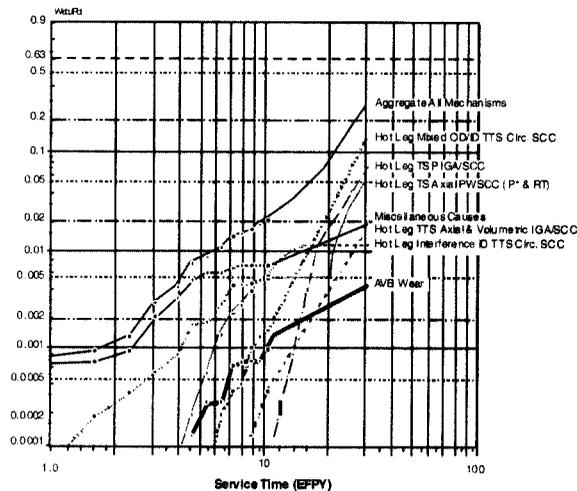
Fig. 2. Cumulative fraction of tubes failed versus service time in Equivalent Full Power Years (EFPY) for seven mode-location cases based on data taken from the steam generators of the Ringhals 4 pressurized water nuclear plant. From Bjornquist and Gorman.<sup>7)</sup>
