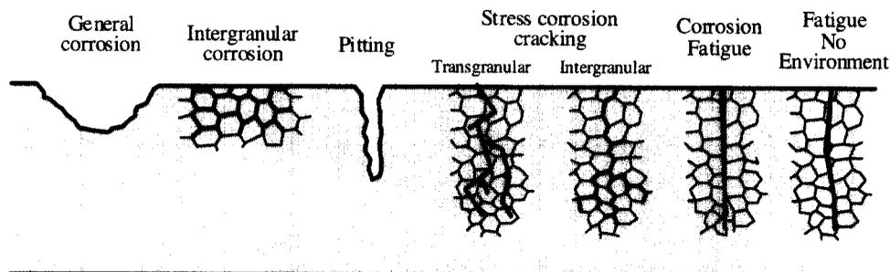
Fig. 8. Views of the intrinsic modes of corrosion.
