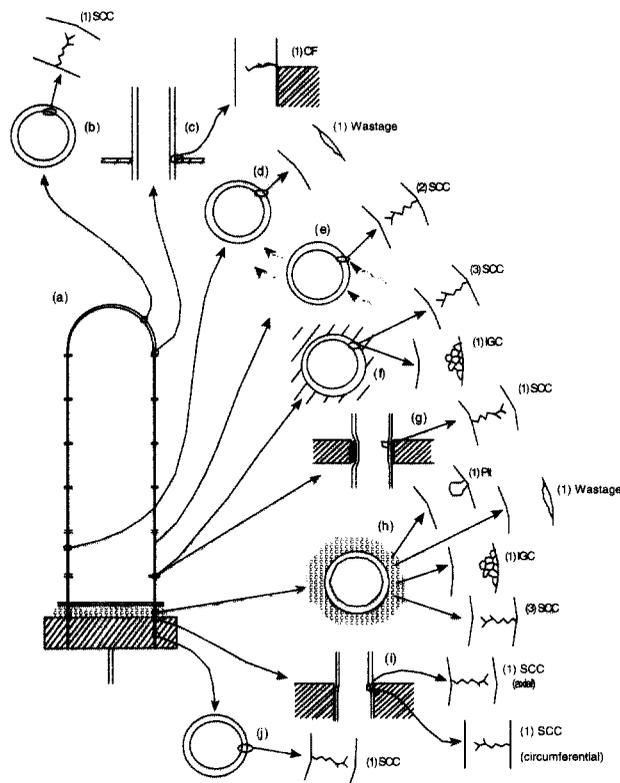
Fig. 5. Schematic view of mode-location cases of corrosion which have occurred in steam generators of pressurized water nuclear reactors. From Staehle.<sup>1)</sup>
