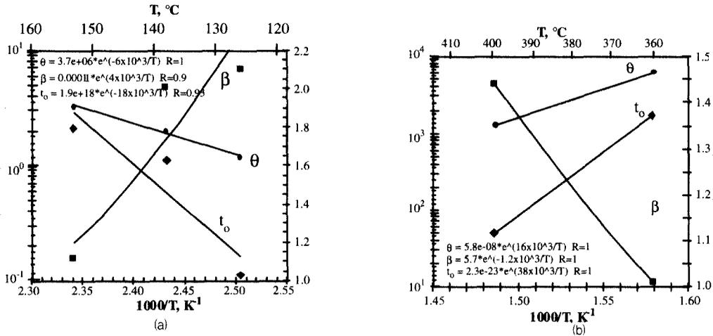
Fig. 14. (a)  $\theta$ ,  $t_0$ , and  $\beta$  versus  $1/T$  for Type 304 stainless steel exposed to concentrated  $MgCl_2$  solutions. Adapted from Shibata.<sup>23</sup> (b)  $\theta$ ,  $t_0$ , and  $\beta$  versus  $1/T$  for the LPSCC of Alloy 600MA exposed to high purity deoxygenated water containing a hydrogen concentration of 10-60 cc  $H_2/kg$   $H_2O$ . Adapted from Webb.<sup>24</sup>
