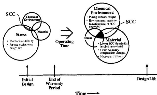
Fig. 1. Schematic view of relative importance of factors contributing to SCC over time from initial design, end of the warranty period, and at the design life. From Staehle.<sup>2)</sup>
