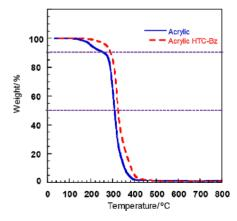
Fig. 9 Thermal weight loss curves of pure acrylic coating and coating containing HTC-Bz.
