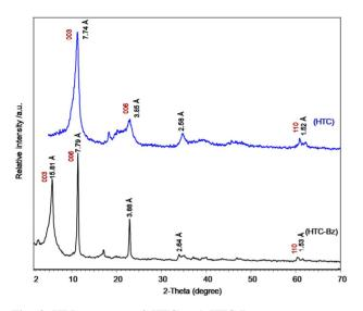
Fig. 2 XRD patterns of HTC and HTC-Bz.
