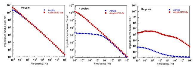
Fig. 5 Impedance diagrams of pure acrylic coatings and acrylic coating + HTC-Bz before and after QUV exposure.
