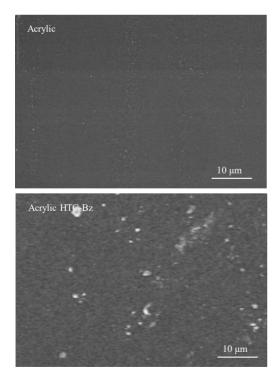
Fig. 8 SEM images of acrylic coating and acrylic coating containing HTC-Bz.
