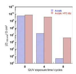
Fig. 6  $|Z|_{\rm 100\ mHz}$  values of blank coating and coating containing HTC-Bz at different exposure times.
