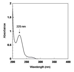
Fig. 4 UV-Vis spectrum of HTC-Bz solution.
