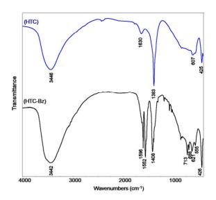
Fig. 3 FT-IR spectra of HTC and HTC-Bz.
